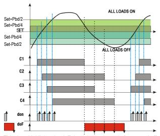
This draw highlights the doF time: the loads are in fact turned off only when the doF time is over.
