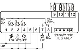
NOTE: The compressor relay is 8(3)A or 16(6)A according to the model. 24Vac supply: connect to the terminals 5 and 6.
