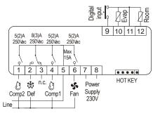
24Vac supply: connect to the terminals 7 and 8. 120Vac supply: connect to the terminals 7 and 8.
