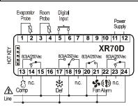
24Vac/dc supply: connect to the terminals 11 and 12. 120Vac supply: connect to the terminals 11 and 12. 230Vac supply: connect to the terminals 11 and 12.
