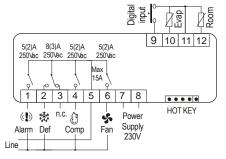
24Vac supply: connect to the terminals 7 and 8. 120Vac supply: connect to the terminals 7 and 8.
