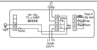
Supply: 120Vac or 24Vac: connect to terminals 5-6 The X-REP output is optional
