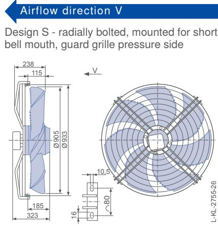
Design S - radially bolted, mounted for short bell mouth, guard grille pressure side
