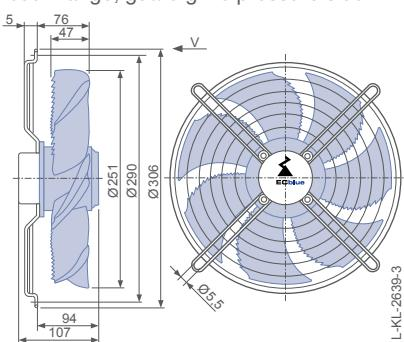
Design H - pipe sockets with a flange, guard grille pressure side
