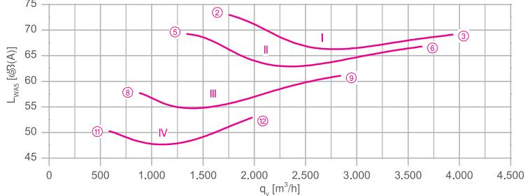
Measured in full bell mouth without guard grille in installation type A according to ISO 5801
