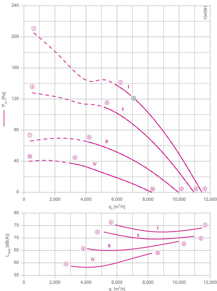
Measured in ZAplus without guard grille in installation type A according to ISO 5801
