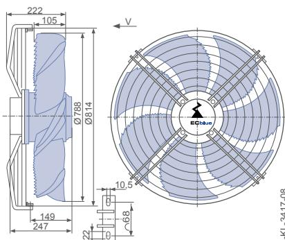
Design I - axial bolted, mounting for bell mouth flange, guard grille pressure side
