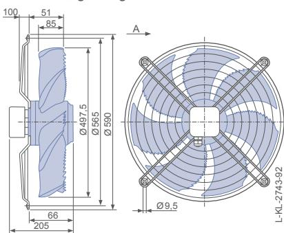
Design W - axial bolted, mounting for short bell mouth, guard grille suction side
