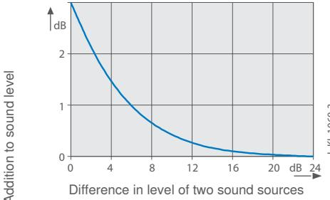
Fig. III: Sound sources of different levels
