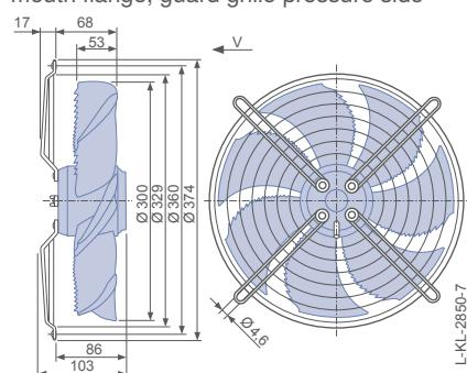
Design H - pipe sockets with a flange, guard grille pressure side
