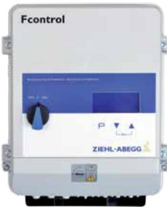
The 1~ Fcontrol frequency inverters with all-pole effective sine filter are available in the version as a temperature control unit. A TFR type temperature sensor (room temperature sensor IP54) is contained in the scope of supply. The frequency inverters control asynchronous motors (external rotor motors, IEC standard motors) gently, requirement-based and energy saving.
