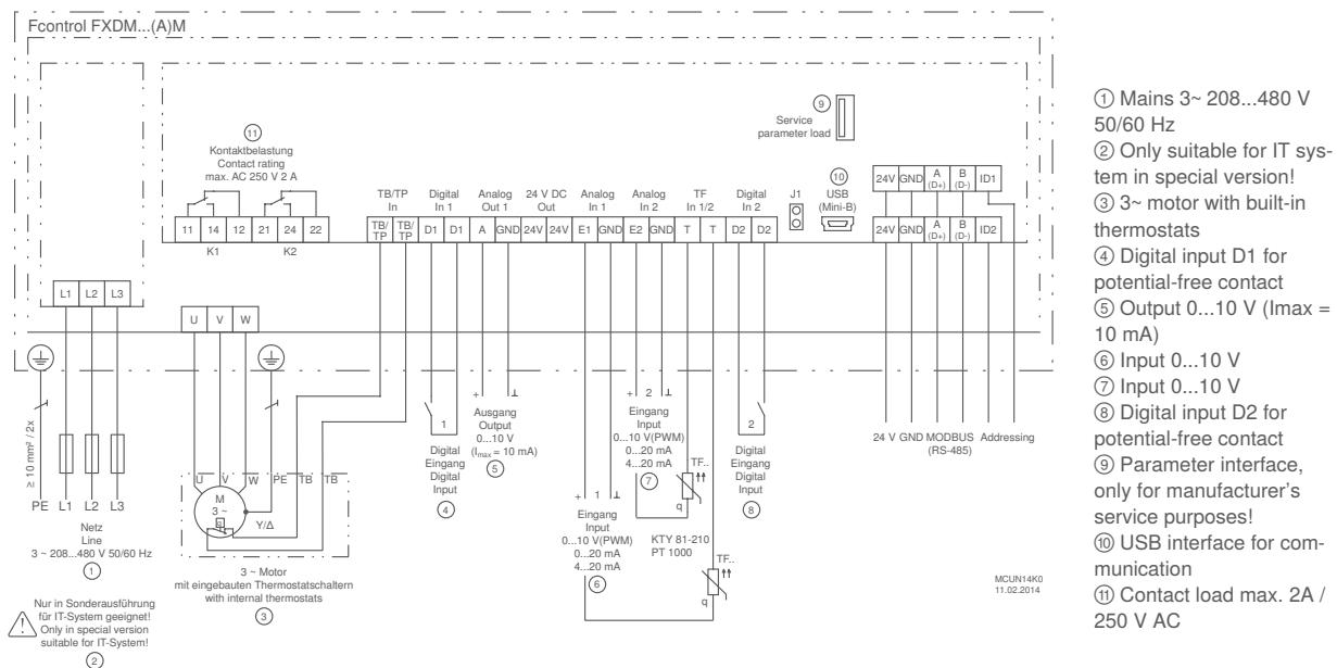
The Fcontrol frequency inverters offer special benefits. Fcontrol have an integrated all-pole active sine filter which ensures a sinusoidal output voltage which is comparable with the normal supply network. This means that the frequency inverters enable reliable, requirement-based, energy-saving control of asynchronous motors (external rotor motors, IEC standard motors) without needing to consider measures that must be observed with standard frequency inverters.
