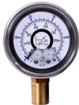
The sensor control module for pressure measures and displays the pressure, for instance in refrigeration circuits. Depending on the desired setpoint and control range, the sensor control module generates 0-10 V to control the EC fan or, for example, a frequency inverter.
