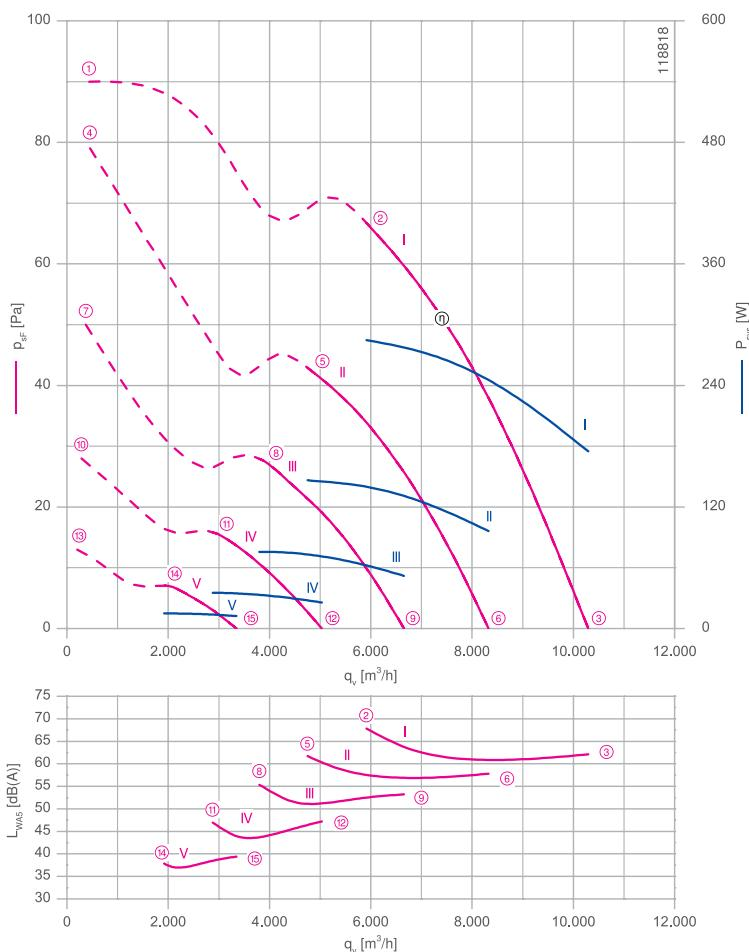
Measured in ZAplus without guard grille in installation type A according to ISO 5801
