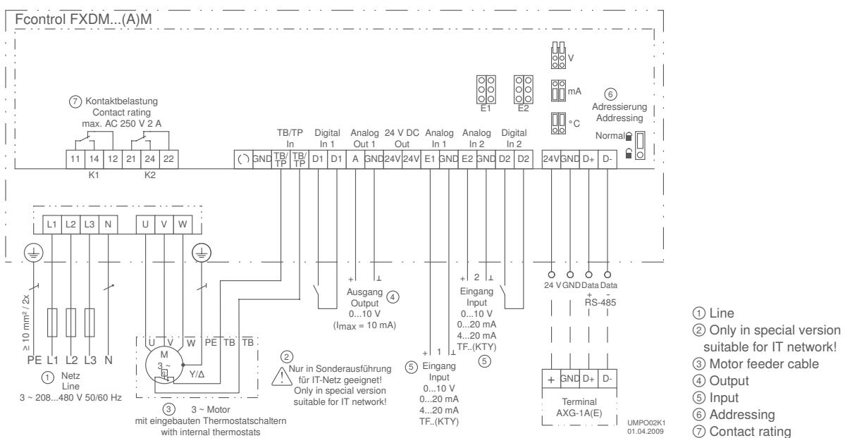
The Fcontrol frequency inverters provide special advantages. Fcontrols have an all pole effective sine filter integrated which provides sinusoidal output voltage that is comparable with the standard mains. That means the frequency inverter enables reliable, demand-oriented and energy-saving control of asynchronous motors (external rotor motors, IEC standard motors) without having to take measures into consideration required by standard frequency inverters.
