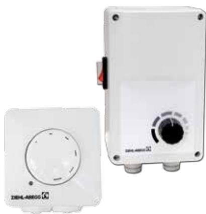
These devices for continuous speed control of one or more voltage-controlled 1~ fans have a knob installed at the front. This knob sets the desired speed. The speed controller starts with maximum output voltage for safe start-up of the fan.
