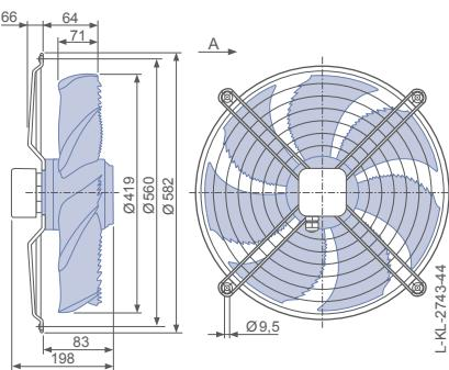
Design D - axial bolted, suspension for full bell mouth, guard grille suction side
